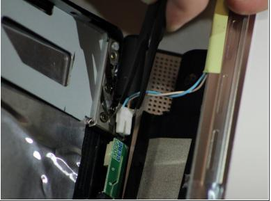
Disconnect the camera connector from the circuit board to completely free the screen.
