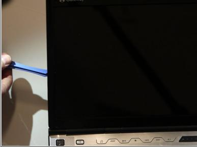
Separate the plastic screen casing from the laptop lid by inserting a plastic opening tool. Complete this step around the top and along both sides of the screen.
