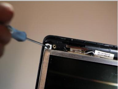
Remove the two 4mm Phillips #0 screws located at the top that fasten the screen bracket to the laptop.
