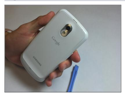
You must open the back of the phone to access the battery. To do this use the plastic opening tools or your fingernail and insert it into the divot.
