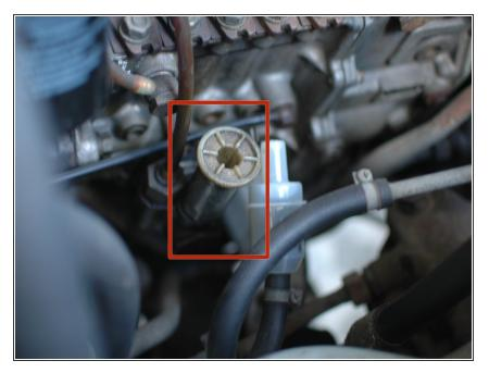
Seen here is the original primer pump on this 1979 300CD. It is an older style that has become prone to leaking after all these years. We are going to replace it with an updated style by Bosch.
