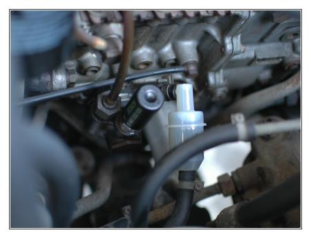
Now screw the new primer pump in by hand as far as you can, then use a wrench (the new ones take a 17mm) to snug it down. There is no need to wrench on it really heavily, just turn it until you feel resistance as the crush washer deforms to create a seal under the pump.
