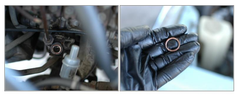
Under the old primer pump will be a copper crush washer. This must be removed before installing the new pump as you'll be installing a new crush washer. Use a small flat blade screw driver to gently push and pry on this washer to remove it.
