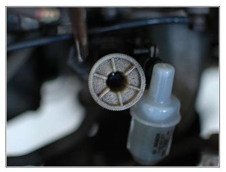
• Note the fuel in the cavity on top of the pump. This pump was definitely leaking. Most of them do these days.
