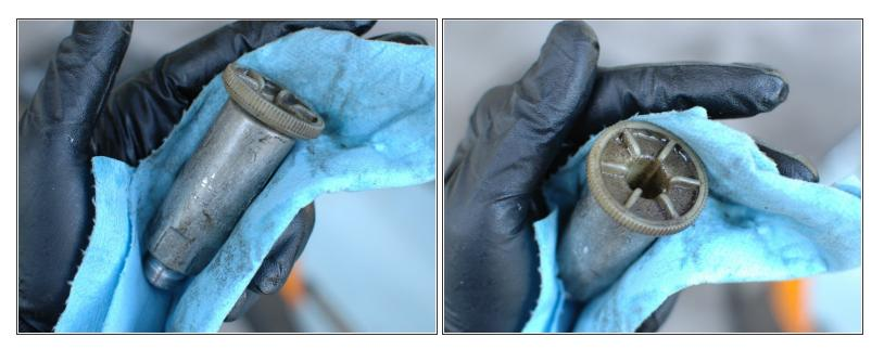
• Here is the old primer pump removed from the car. You can see the minimal damage that the vice grips did to the body of it. Also, in the second picture, you can see how wet, discolored, and dirty the pump knob is. This is from leaking fuel.
