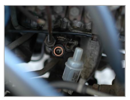
Carefully use a shop towel to wipe any dirt out and away from the opening in the lift pump, then install the new crush washer.
