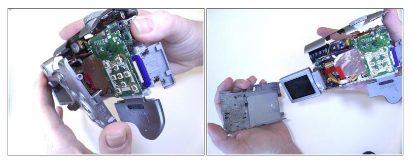
• Gently pull the back panel to separate it from the camera.
