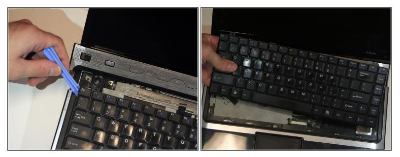
• Gently pry up on the corners of the keyboard with the plastic opening tool to free the keyboard.
