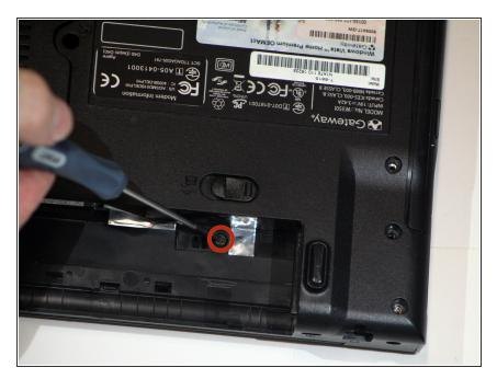
Remove a 4mm Phillips #0 screw just beneath the battery that holds the speaker cover panel.
