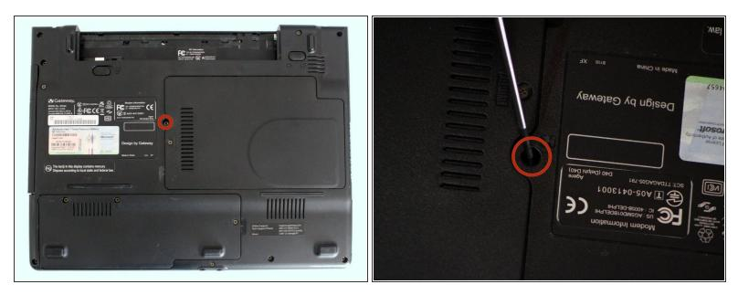
• Remove the 4mm Phillips #0 screw that secures the keyboard.
