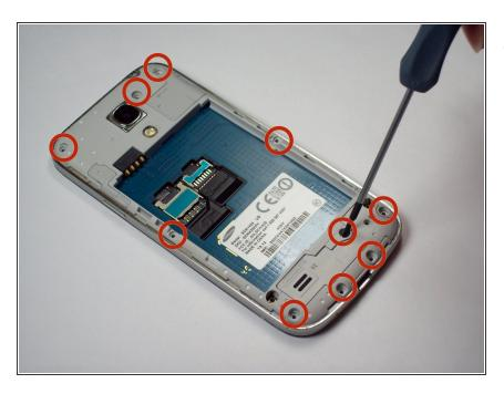
In the back, there are 10 screws with a, which have to be removed with a small Phillips screwdriver tool.
