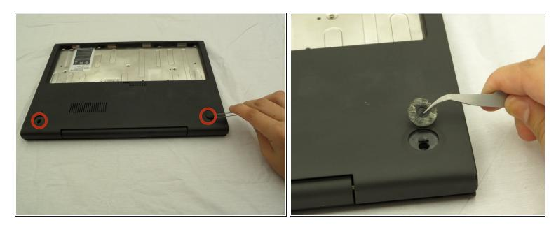
• Using a pair of tweezers, remove the two rear rubber feet to expose two hidden screws.
