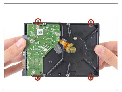
Remove the four 8.1 mm T8 screw posts from the hard drive, and transfer them to the replacement drive enclosure.
