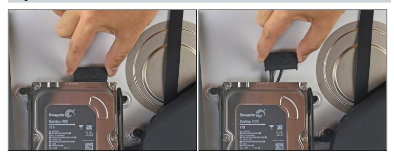
• Pull straight up on the SATA combo cable to disconnect it from the drive.
