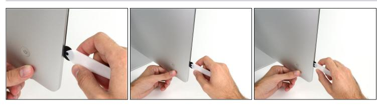
Starting on the left of the display, near the power button, insert the iMac Opening Tool
