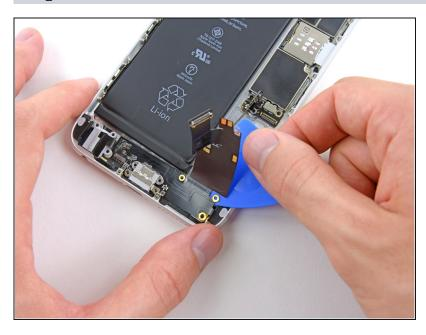
Insert the pick underneath the right bottom corner of the Lightning connector and headphone jack cable.
