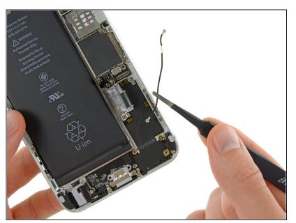
• Lift and remove the antenna connector out of the iPhone.
