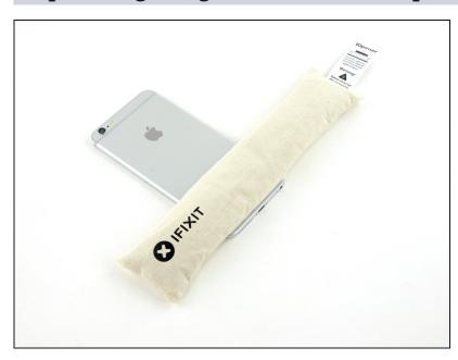
i The next step requires peeling the Lightning connector and headphone jack cable that is affixed to the inside of the rear case with mild adhesive. We highly recommend using an iOpener to heat the lower backside of the rear case.
