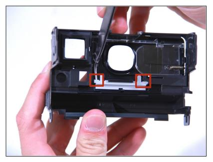
Once you have the face plate removed the first thing to do is pry off the slider (the light grey bar near the bottom). The easiest way to accomplish this is to place the tweezers where the red circles are to pop the piece out.
