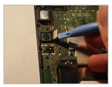
Gently lift up on the metal connector plate.
