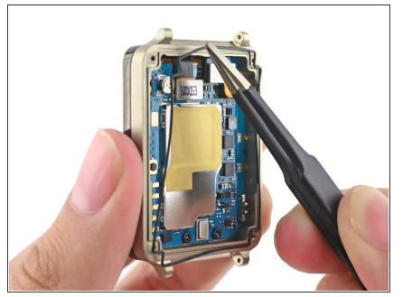
Use a pair of tweezers to remove the gasket that lies embedded in a groove that runs around the perimeter of the front half.
