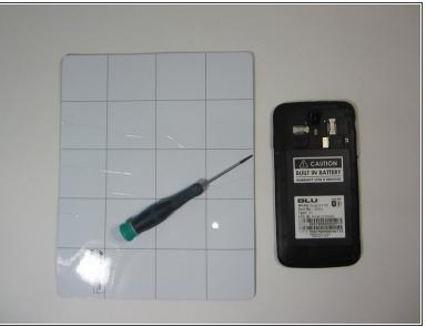
With your back panel already removed from the previous guide you'll need to acquire a Philips head screw driver size (PH00)
