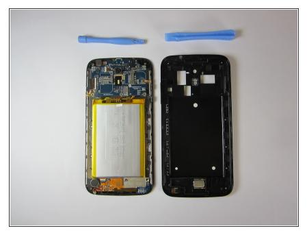
At this point your battery, motherboard, rear camera, and front camera should all be readily available for fixing. Happy fixing.
