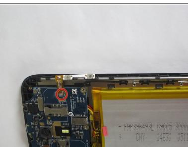
Using the tweezers lift the volume buttons and unsolder the buttons connection.
