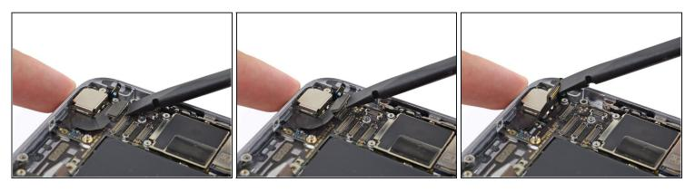
• Use the flat end of a spudger to lift the camera cable connector straight up out of its socket on the logic board.
