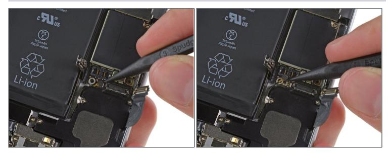
• Use the point of a spudger to lift the antenna cable connector up off of its socket on the logic board.
