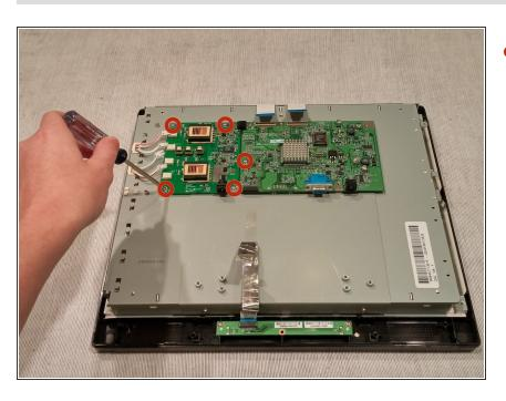
Unscrew the 5 screws holding the Power Supply and Video Display boards.
