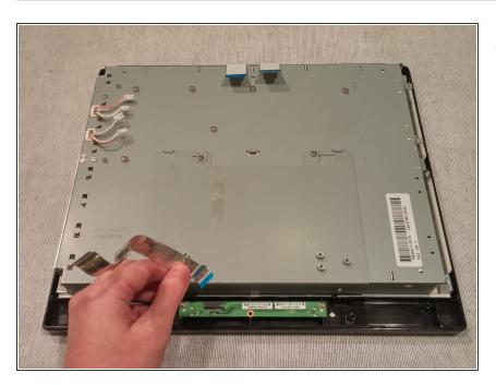
Remove the Flat Flex Cable from the Power Button Circuit board.
