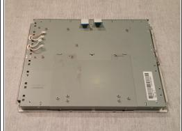
Grasp, lift, and remove the LCD Module from the front panel.
