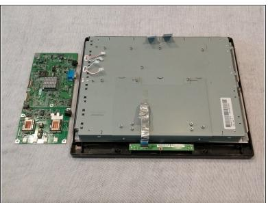
Lift and remove the joined Power Supply and Video Display boards.
