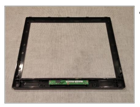
The final product with the LCD Module removed.
