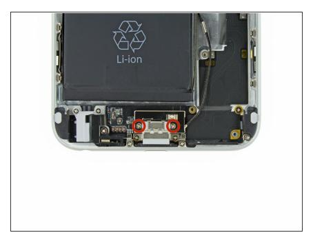
Remove the two 3.3 mm Phillips #00 screws securing the metal bracket to the Lightning connector assembly.
