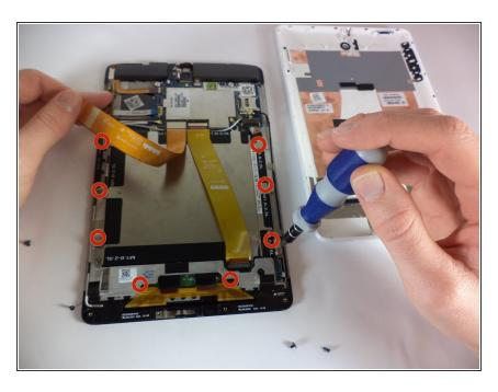
Remove all screws from the sides of the battery
