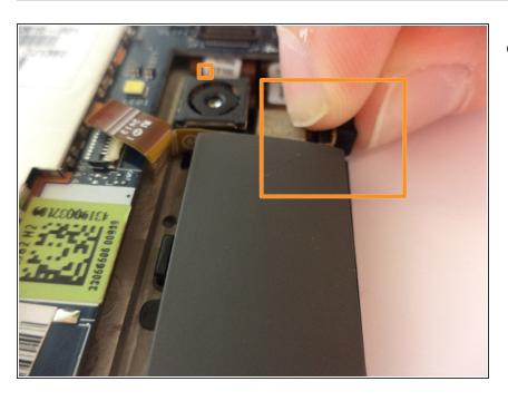
Release the ZIF connector to which the microphone cable is attached
