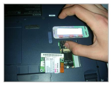
Push your new clock battery into place using your thumb or index finger at the same place where you removed the old clock battery.
