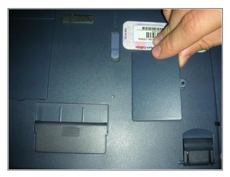
Remove the capsule cover to reveal the computer chip.
