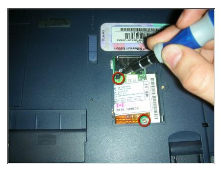
Carefully replace the computer chip and secure the two screws using your Phillips #1 screwdriver by turning the screwdriver clockwise.
