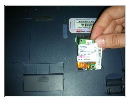
Carefully remove the computer chip and set it aside.
