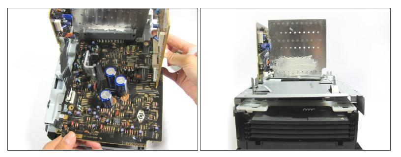
• Slide the mainboard away from the black and green circuit board and then up.
