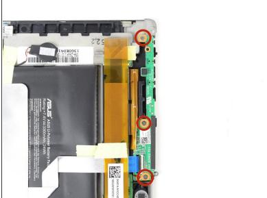
Use a Phillips #00 Screwdriver to remove the three 3 millimeter screws securing the buttons to the back panel.
