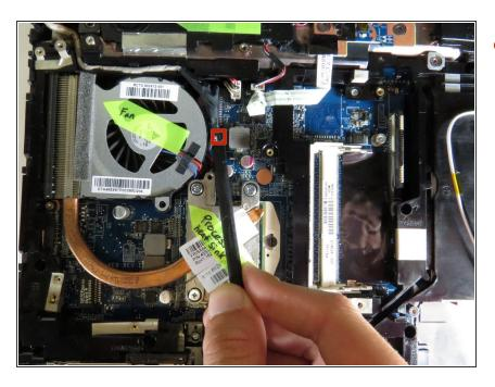
Disconnect the red, black, and blue ribbon cable connector using the black spudger.
