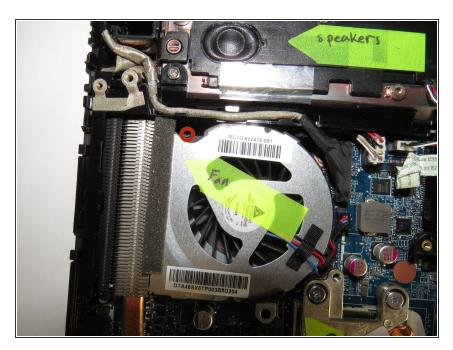
Unscrew the one (2.0 mm Phillips) screw holding in the fan.
