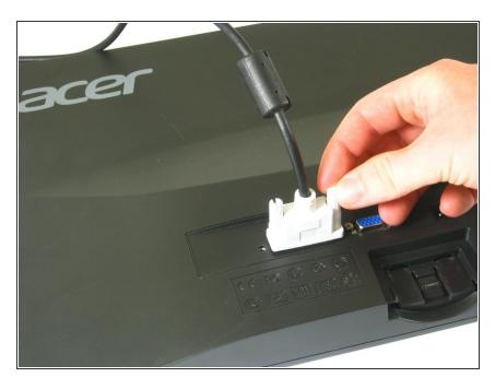
Unscrew the fasteners to the DVI input connector.
