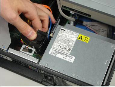
• Grab the plastic casing and pull out the bundle of cables from the side of the power supply unit.
