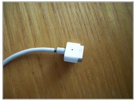
• This is a hyper extended end of a magsafe. It is no longer working due to the wire having pulled apart.
