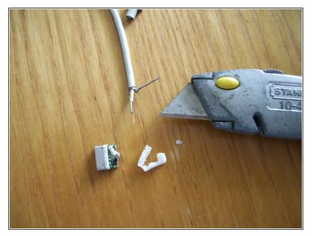
I used a utility knife to cut the nice white cover off the tiny printed circuit board. There is a molded plastic cover similar to hot glue which had to be stripped off the PCB.
