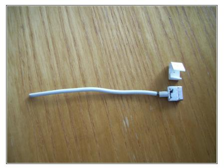
Use wire cutters to cut the wire of the magsafe some distance back from the magnetic end. I cut about 4 inches back. You can get much closer like maybe an inch, as you will see in the next step.
