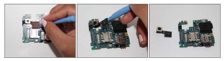
• Using the opening tool, pry up the camera attachment from the motherboard.
