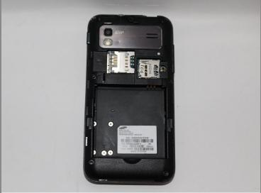
• Remove the seven screws from backplate using the #00 screwdriver.
