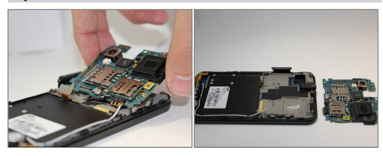
• Lift the motherboard out of the base of the phone.
