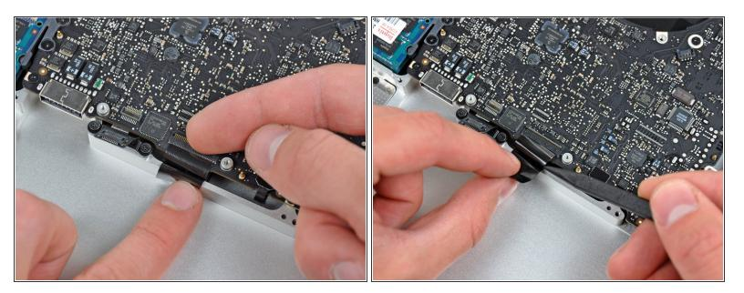
Use your fingernail to carefully flip up the keyboard ribbon cable retaining flap.
