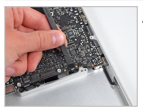
Use the flat end of a spudger to pry the battery indicator cable connector up out of its socket on the logic board.
