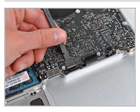
Use the flat end of a spudger to pry the trackpad cable connector up out of its socket on the logic board.
