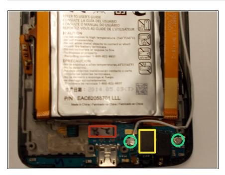
Disconnect the 2 connectors. The LCD connector (red color coded) and the Digitizer (yellow color coded). Together with these 2, remove the 2 antenna connections (green color coded) also.
