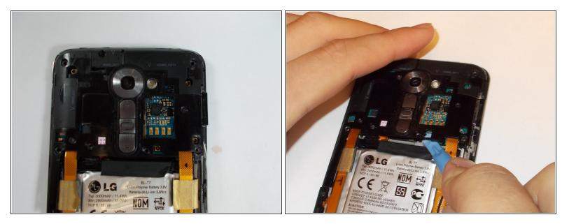
• After all visible screws have been removed use the spudger to pop off the top plastic cover.
