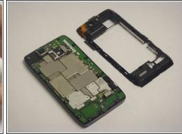
Separate the housing from the motherboard.
