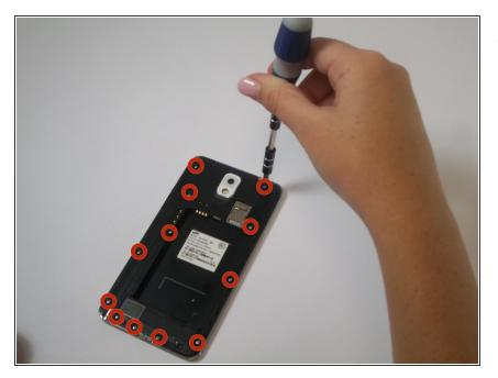
Remove the twelve 4mm Phillips #00 screws from the back chassis.
