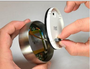
Pinch the gray 20-pin connector with your fingers and pull directly away from the display.
