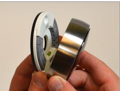
Grasp the display's metal outer ring with your fingers and pull directly away from the wall.
