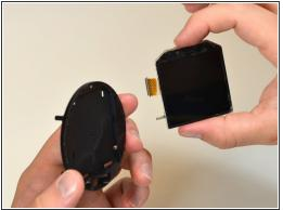
Pull the LCD screen away from the plastic frame gently using your fingers.
