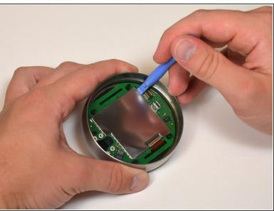
Remove the EMI shield from the motherboard using the plastic opening tools.
