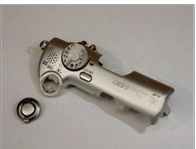
Trigger button should fall out
