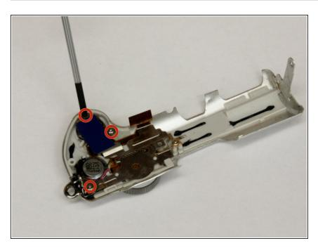
Remove the two screws holding down the metal frame using the Phillips #00 screwdriver
