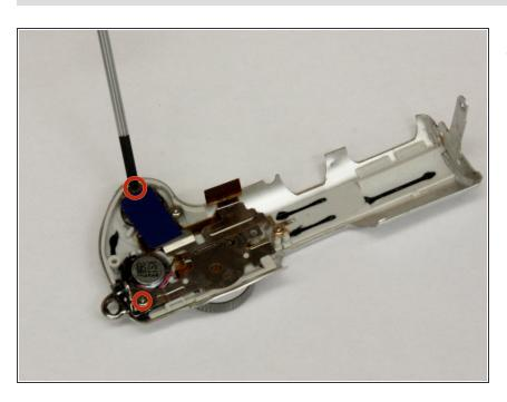
Remove the 2 mm screws from the metal plate.
