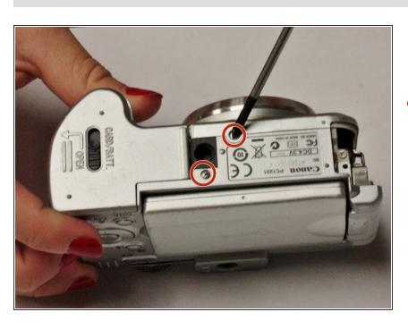
Remove the two indicated .2mm screws using a Phillips #00 screwdriver.
