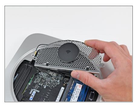
Remove the antenna plate from the mini.
