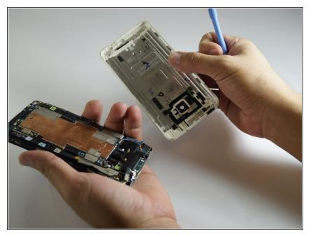
Pry the back open once loose and lift. The back panel will come off with time.
