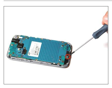
Remove one Phillips 3.93 mm screw from bottom center of the phone.
