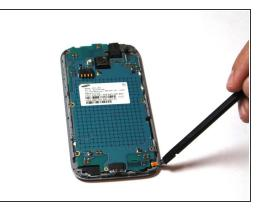
Carefully disconnect 3 ribbons at the shown location. To remove, place tool under the ribbon and pull slowly to avoid tearing.
