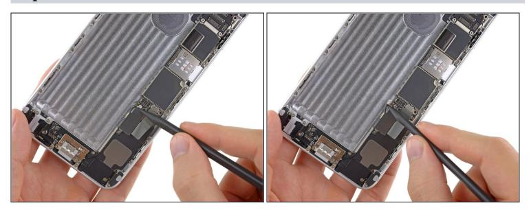
• Use the tip of a spudger to disconnect the interconnect antenna cable from its socket on the logic board.
