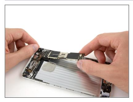
Carefully raise—but do **not** remove—the logic board,
