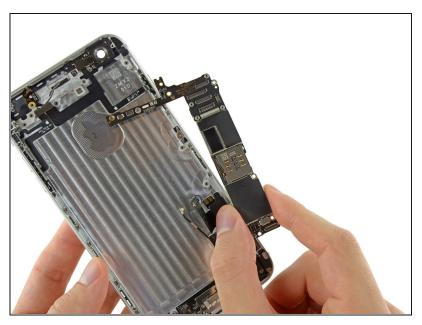
• Lift and remove the logic board out of the iPhone.
