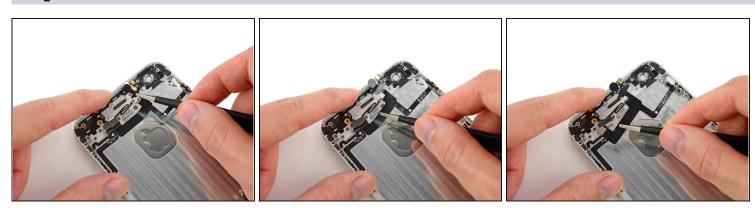
• Continue gently peeling the power button cable off the rear case and remove it from the iPhone.
