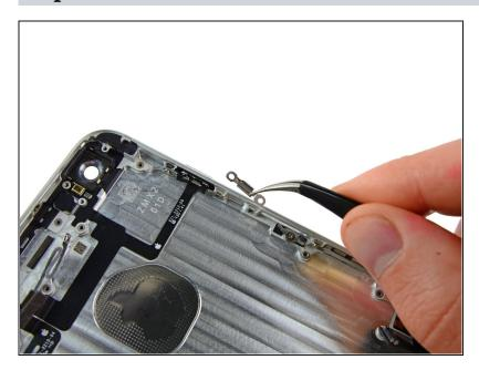
Grasp the power button cable bracket with a pair of tweezers and remove it from the iPhone.
