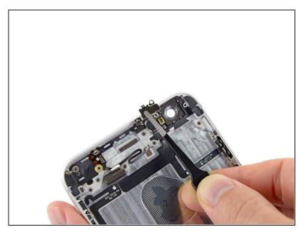
Carefully grasp the bracket with a pair of tweezers and remove it from the iPhone.
