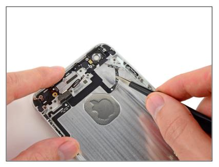
Pull the power button switch out of its recess on the rear case with a pair of tweezers, and begin carefully peeling the power button cable from the rear case.
