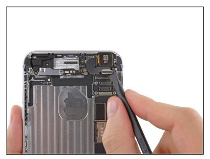
Use the flat end of a spudger to disconnect the rear-facing camera connector from its socket on the logic board.
