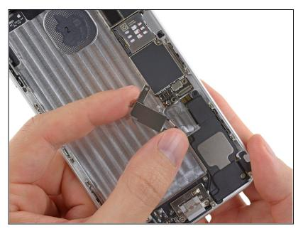
• Lift and remove the vibrator out of the iPhone.
