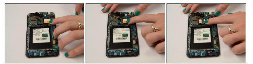
• Remove or replace SIM Card by pushing into metal slot above the battery holder.
