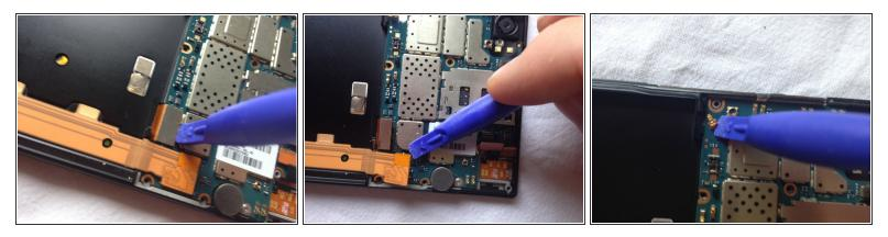
• Let's unclip screen ribbon then dock ribbon. Finally the antenna clip.
