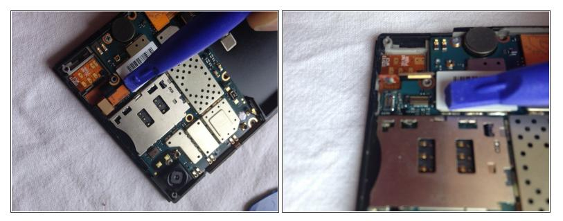
• Unclip the upper screen ribbon. Then, unclip the jack ribbon.
