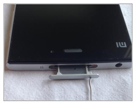
• To start, it is needed to remove the SIM tray. You will find 2 (two) small Phillips screws. Make sure to understand that opening the orange one will void the warranty.
