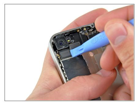
Use an iPod opening tool to carefully lift the rear camera connector up off its socket on the logic board.
