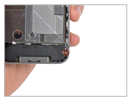
Remove the single 2.4 mm Phillips screw securing the speaker enclosure to the side of the inner frame.
