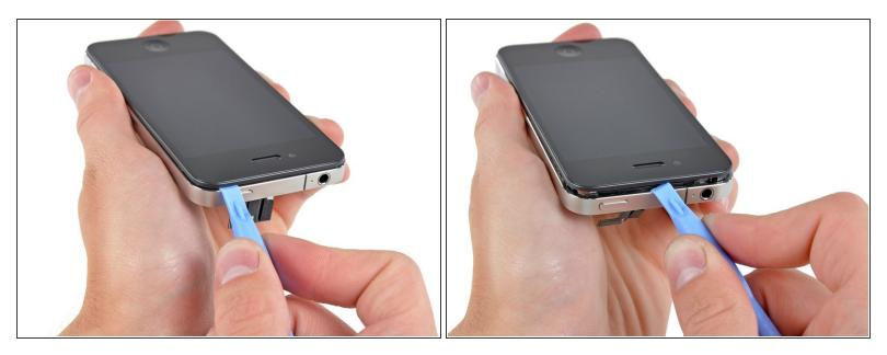
• Carefully insert the edge of an iPod opening tool between the rubber bezel around the front glass panel and the steel inner frame.
