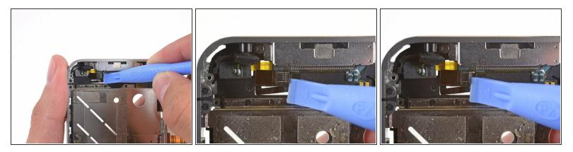
Use the edge of an iPod opening tool or your fingernail to lift the home button ribbon cable retainer.
