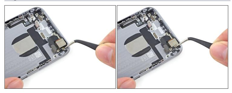
• Carefully remove the antenna interconnect cable from the rear case.
