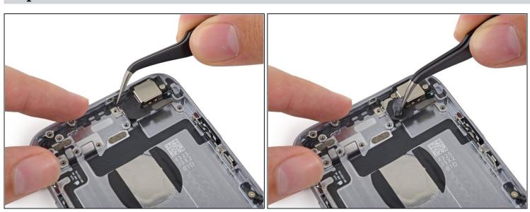
• Remove any tape covering the upper left rear-facing camera screw.
