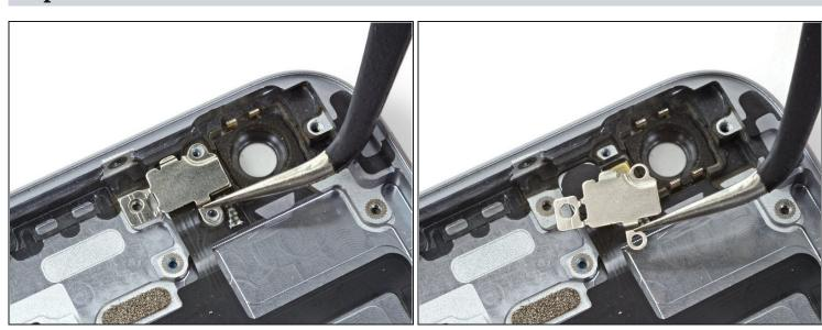
• Remove the flash bracket from the rear case.
