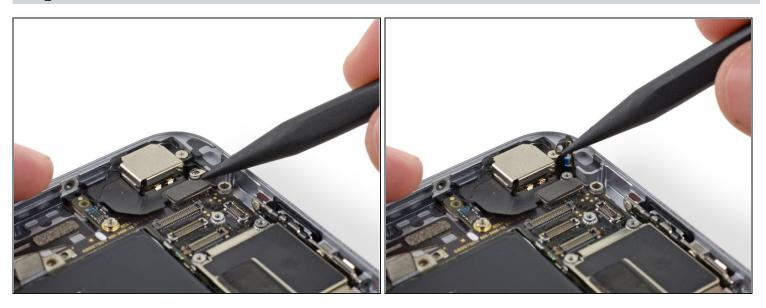
Use the point of a spudger to fold the antenna interconnect cable up out of the way of the logic board.
