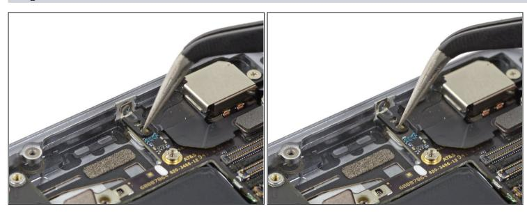
• Remove the angled logic board bracket.
