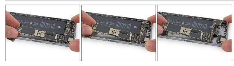
Lift the battery connector end of the logic board and pull it up and out of the rear case.
