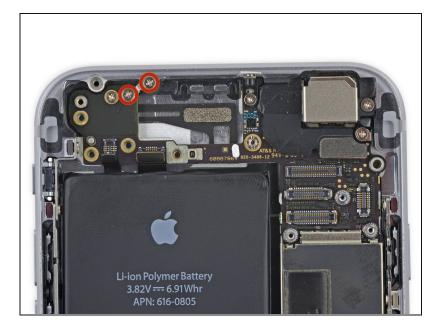
Remove the two 1.6 mm Phillips screws from the grounding bracket.
