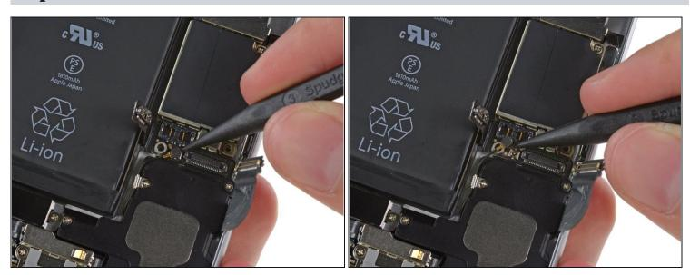
• Use the point of a spudger to lift the antenna cable connector up off of its socket on the logic board.
