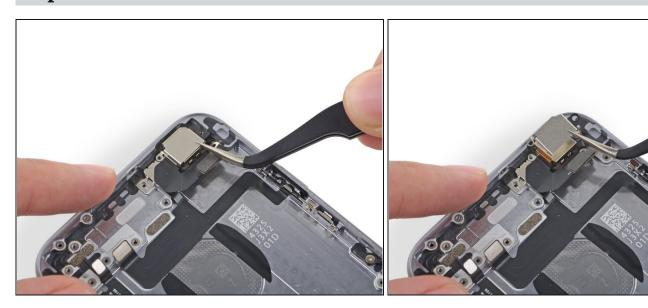
• Remove the rear-facing camera bracket.
