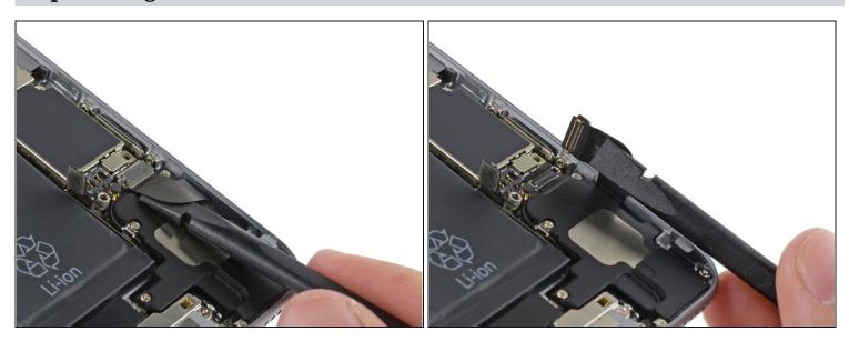
• Use the flat end of a spudger to disconnect the Lightning connector assembly cable and fold it out of the way of the speaker.
