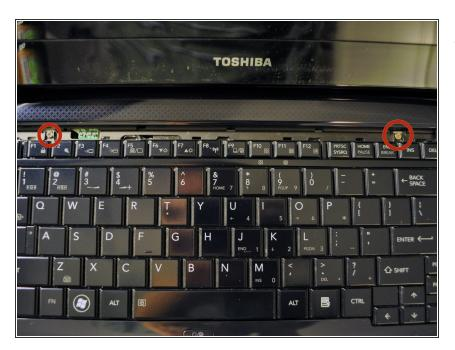
Remove the two screws securing the keyboard to the chassis.
