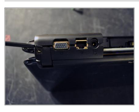
Carefully work a spudger in the crack at the back of the laptop and separate the small rubberized
