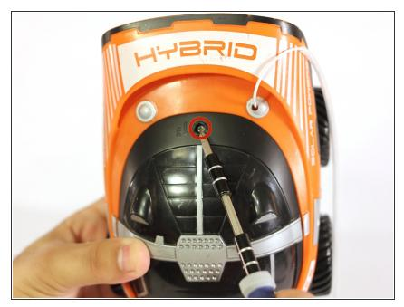
First, completely loosen the 9.6 mm Phillips #2 screw on top. There is a plastic washer that holds the screw to the top cover, so it will not need to be taken out.
