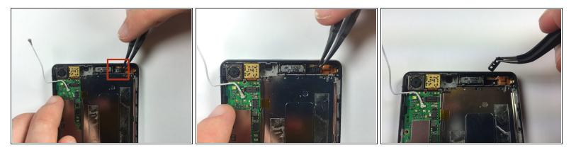
Use tweezers to lift the rubber alignment tab out of its frame.
