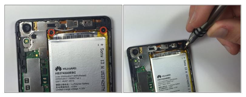
Push down the yellow plastic lining at the top of the battery and remove the two 2.5mm Phillips #000 screws.
