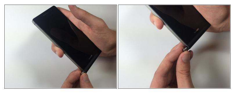
• Pull and twist the pin near the bottom left-side of the phone to remove it from the headphone jack.
