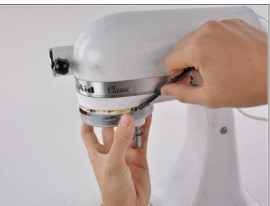
Using a spudger, gently pry off the aluminum drip ring.
