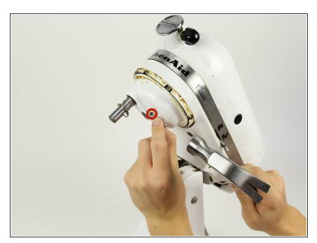
Using a 4 mm pin punch and hammer, hammer the pin until it is dislodged from the planetary gear cover.
