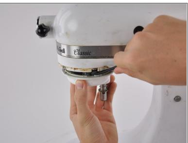
Using a spudger, pry the planetary gear cover from the mixer shaft.
