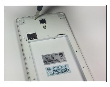
With the 3.6 mm Phillips screwdriver, remove the three newly exposed 3.6mm Phillips screws.
