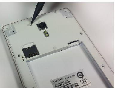
Remove the three circular rubber screw covers on the back of the phone by slipping the spudger into the border between the rubber cover and the chassis. In one motion, pry the stopper out of the hole. This can take some force.
