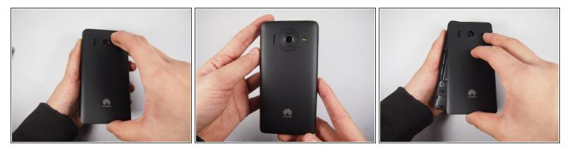
• Remove the rear cover on the back by pulling up on the gap located at the bottom of the phone.
