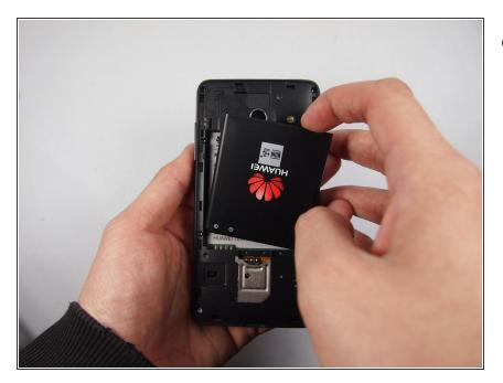
Lift the battery with your finger up and out to remove the battery for replacement.
