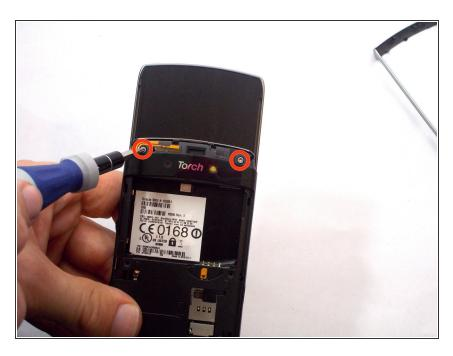
Once you remove the rim cover, you should find two more screws on the top. Unscrew them using the T6 screw driver.
