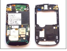
• Use the plastic removal tool to remove the entire back cover.
