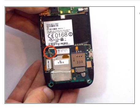
Unplug the black antenna wire from the logic board.
