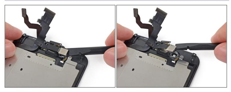
• Lift the front-facing camera out of its recess in the front panel.
