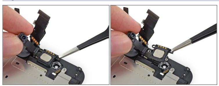
Holding the front-facing camera out of the way, remove the earpiece speaker from the front panel.
