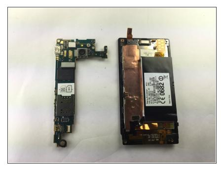
Use the spudger and slide it under the top left of the board then lift the board straight up. The board should come up very easily.
