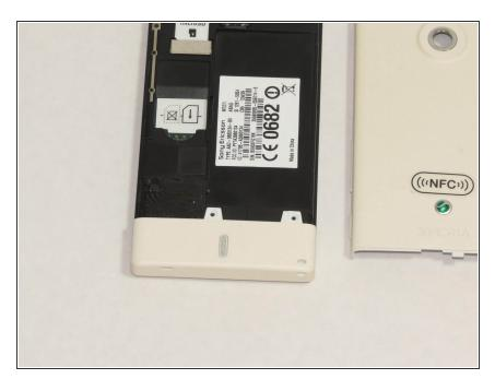
Push on cover away from you. You should hear a snap or pop. This will let you view the battery and sim/sd card slots. Then lift the cover off.
