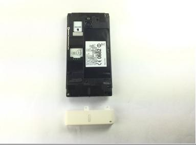
Pry off the bottom white cover by using the opening tool as a lever.
