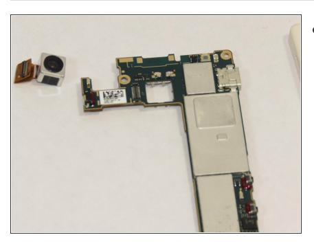
Pick up board and remove camera module. The module should seem to just pop out.
